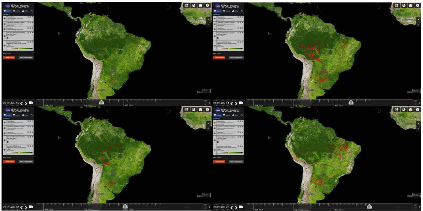
Fig. 1. Satellite images from the NASA's Earth Observing System Data and Information System (EOSDIS) from July 15 to August 28, 2019, showing the MODIS wildfire and Thermal Anomalies layer, able to identify active wildfire and thermal anomalies (red points). The MODIS wildfire and Thermal Anomalies product is available from the Terra (MOD14) and Aqua (MYD14) satellites as well as a combined Terra and Aqua (MCD14) satellite product. The sensor resolution is 1 km, and the temporal resolution is daily. The thermal anomalies are represented as red points (approximate center of a 1 km pixel) in the Global Imagery Browse Services (GIBS)/Worldview. Also, as a base layer, the MODIS Normalized Difference Vegetation Index (NDVI). The index is calculated based on how much red and near-infrared light is reflected by plant leaves. The index values range from -0.2 to 1 where higher values ( 0.3 – 1 ) indicate areas covered by green, leafy vegetation, and lower values ( 0 – 0.3 ) indicate areas where there is little or no vegetation. The MODIS rolling 8-day NDVI layer is available as a near real-time, rolling 8-day product (MOD13Q4N) from the Terra satellite. It is created from a rolling 8-day land surface reflectance product, MOD09Q1N. The sensor resolution is 250 m, imagery resolution is 250 m, and the temporal resolution is an 8-day product which is updated daily. Available at: https://worldview.earthdata.nasa.gov/ . (For interpretation of the references to colour in this figure legend, the reader is referred to the Web version of this article.)
